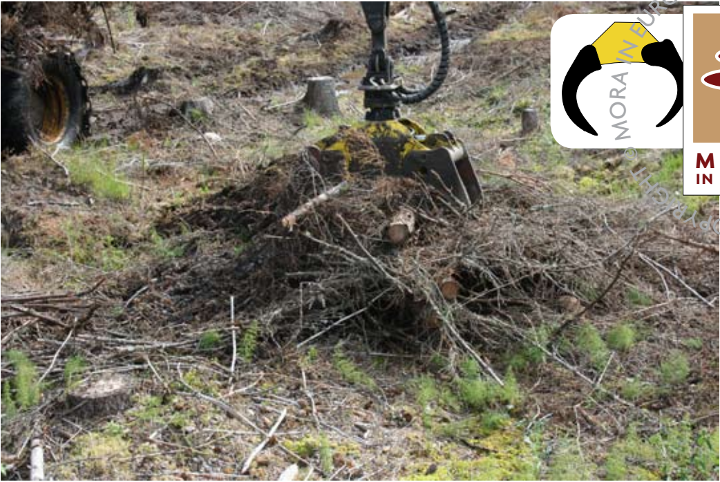
The operator grapples the GROT with the intention of not letting the grapple arms dig down into the ground surface. He grapples “carefully” so that the grapple is not closed more than necessary.
